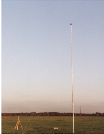
Fig. 2: The receiver set: a microphone with a windscreen on a mast at 12 m (left) or on a tripod at 2 m (right) above the ground.
