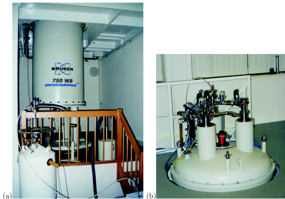
Fig. 1: 17.64 T magnet of the AVANCE 750 at the lower level of the lab (a) and at the upper level (b).
