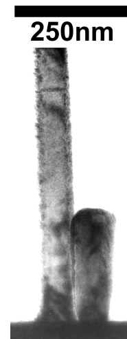
Figure 7.42: Bright field TEM-image of a lateral GaAs/GaN-nanoheterojunction.
