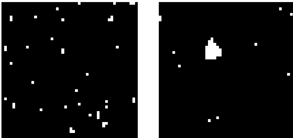
Figure 10.2: Two snapshots of a L = 50 Ising system at the same value of the magnetisation. Left: Evaporated system, a large number of very small bubbles exists (1 to 3 spins). Right: Condensed system, a single large droplet that has absorbed nearly all small bubbles.
