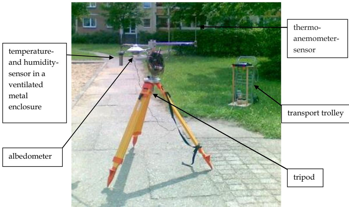
**Figure 1:** *Measurement setup, positioned at a measuring point in Leipzig-Paunsdorf.*
