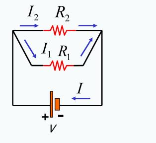
$$I = I_{1} + I_{2} \qquad V = I_{1}R_{1} = I_{2}R_{2}$$
