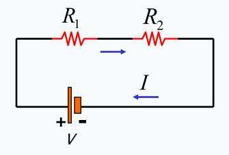
$$V = V_1 + V_2 = IR_1 + IR_2$$
