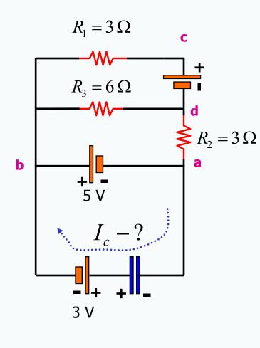
Adding an open circuit does not affect currents in other parts of the circuit.
