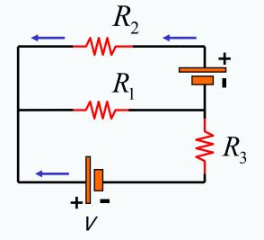
When any closed loop is considered, the sum of the changes in electric potential must be zero.
