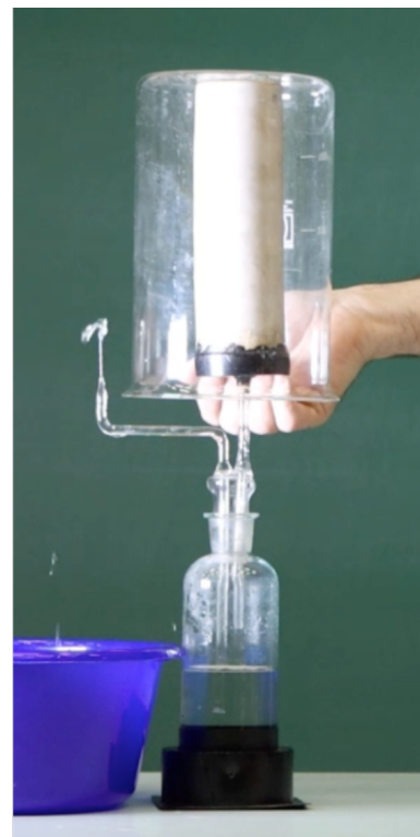
Figure 1.21: Pressure created due to flux imbalance of He and air through a porous membrane. ©Axel Märcker, UL
