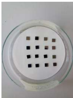
Figure 34: Set of silicon wafers coated with PMMA
