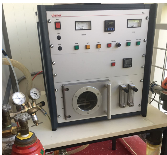
Figure 3.6: Plasma chamber. Note the bottle of oxygen at the left of the picture.
