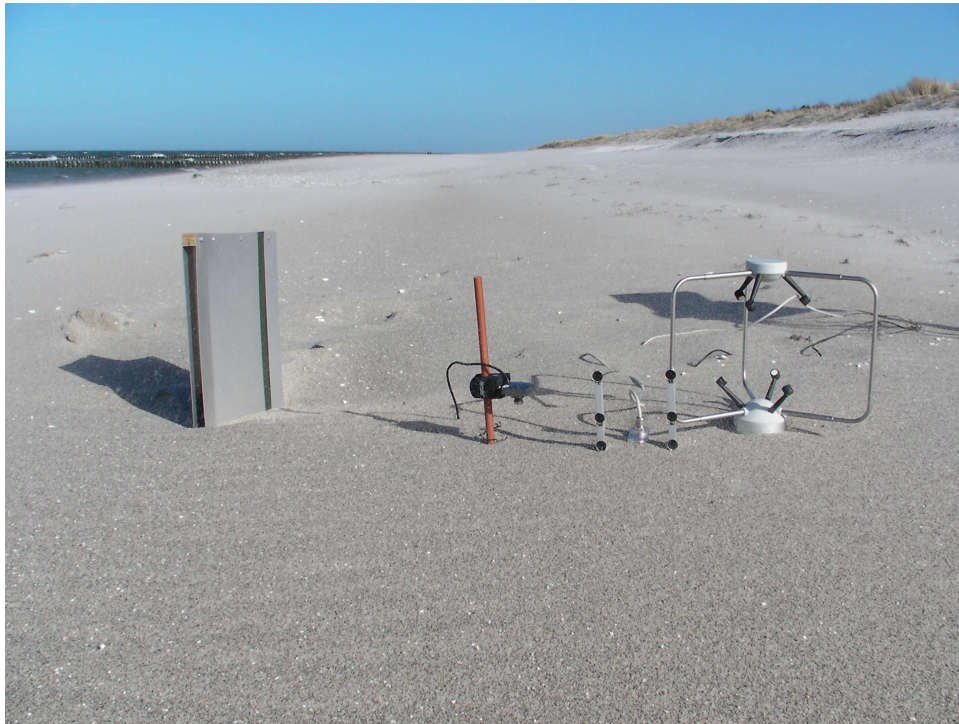
Fig. 3: The instrument array. From left to right: Guelph sand trap, web cam, microphone array of six microphones (work as Saltiphones), and sonic anemometer (buried).
