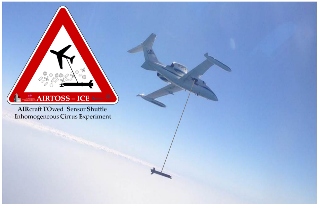
Fig. 1: Learjet with towed AIRTOSS (AIRcraft TOWed Sensor Shuttle). Picture was taken during the test flight from chaser plane.
