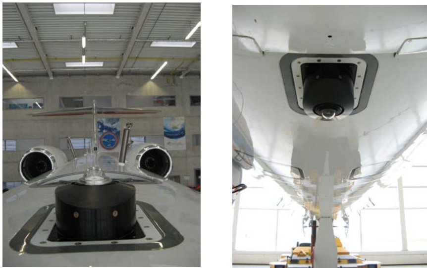
Fig. 2: Sensors for SMART on top (left) and bottom (right) of HALO
