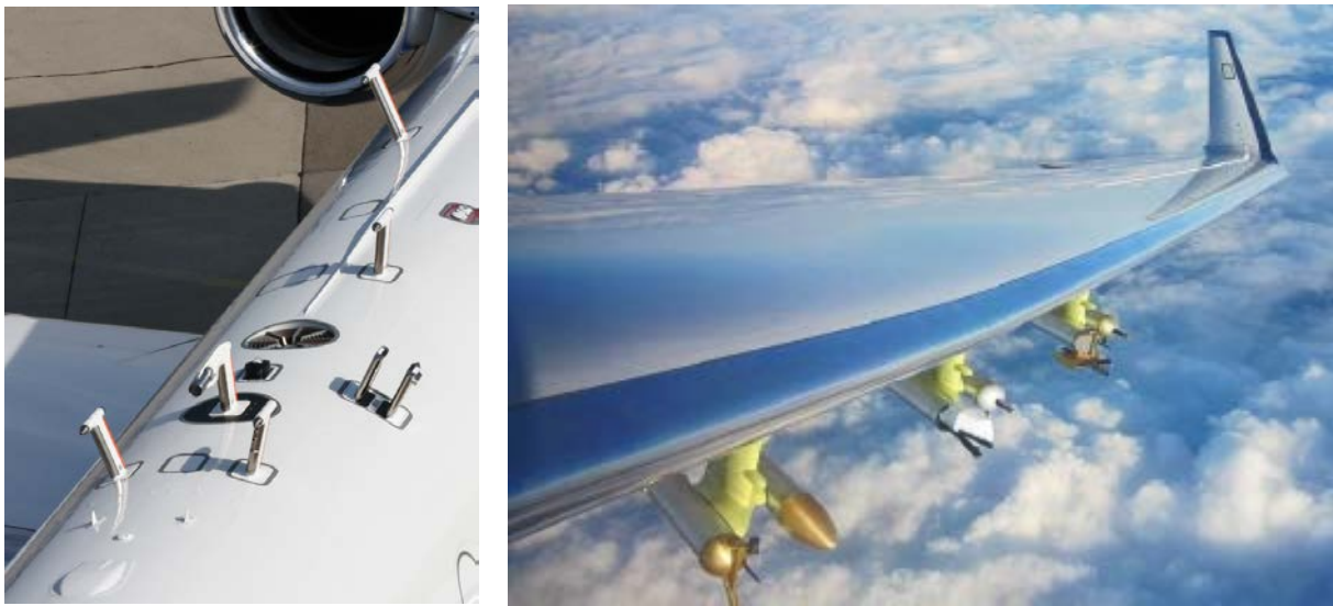
Fig. 3: Inlets on top side of HALO (left) and PMS-carriers below the wings (right)
