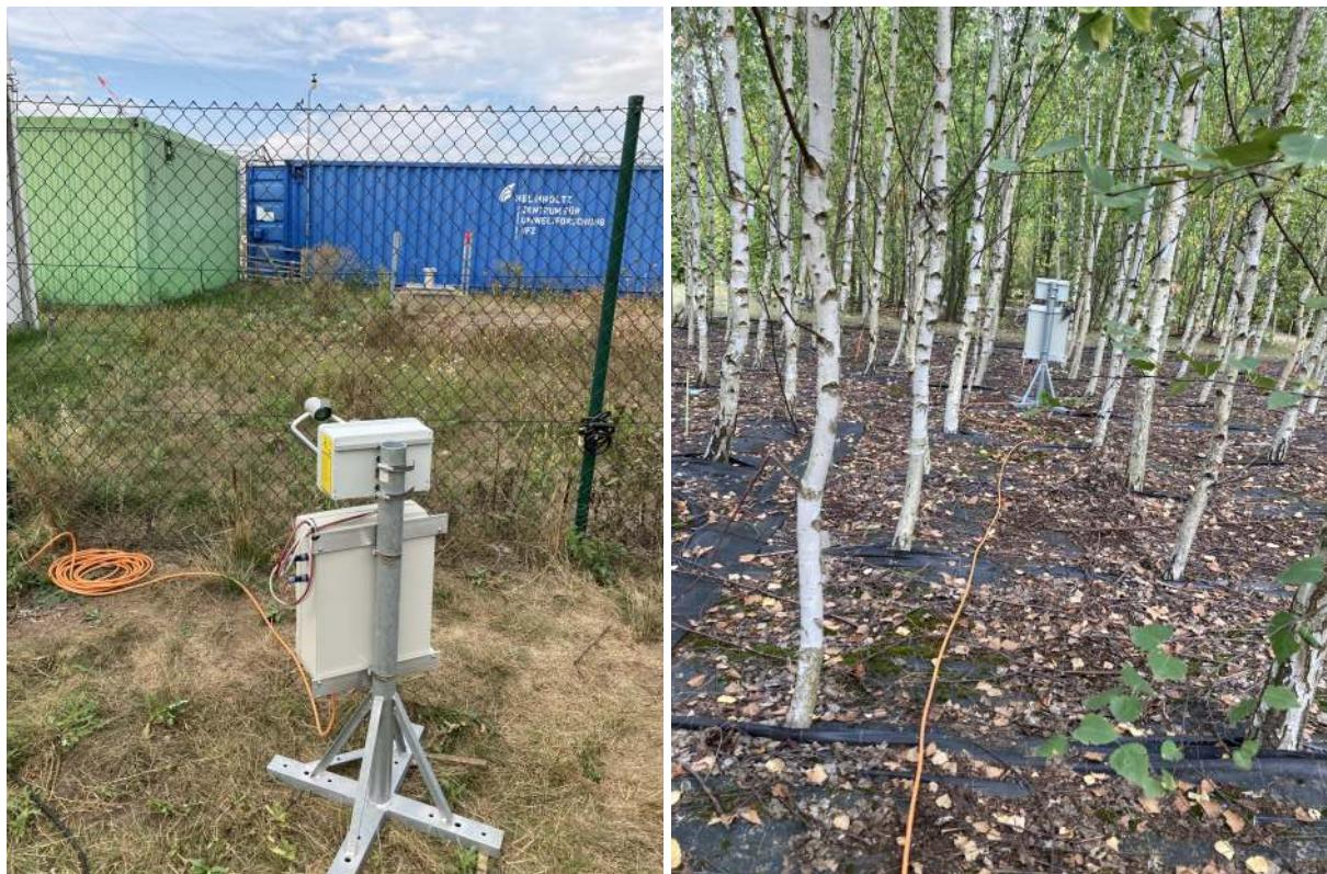
Figure 1: Disdrometers during the measurement campaign, on the left the disdrometer in the open land, on the right the disdrometer under trees in a plot of birch (*Betula pendula*). Images by Andreas Foth.
