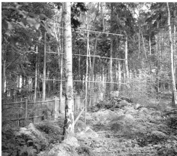
Figure 1: Left: Transmit antenna. In the foreground the trench to carry the feeder cable is still open. Right: Transmitter (right rack) and receiver unit (left rack) installed on a table.
