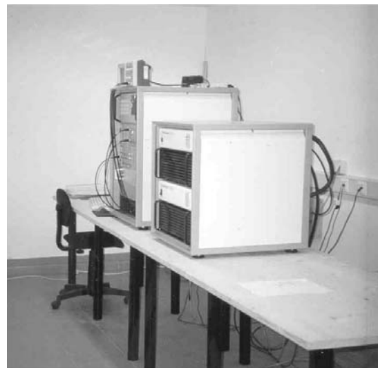
Figure 1: Left: Transmit antenna. In the foreground the trench to carry the feeder cable is still open. Right: Transmitter (right rack) and receiver unit (left rack) installed on a table.
