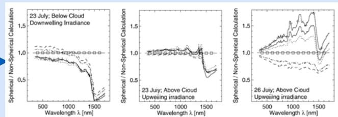
Fig. 5: Ratio of calculated irradiances assuming spherical and nonspherical ice crystal shapes. (a) downwelling irradiances for the flight level of the Twin-Otter (3.6 km,  $\theta_s = 78^\circ$ ) below the cloud on 23 July; (b) and (c) upwelling irradiances for the flight level of the ER-2 (20.7 km,  $\theta_s = 78^\circ$  (b) and 19.2 km,  $\theta_s = 21^\circ$  (c)) above the cloud on 23 July (b) respectively 26. July (c). The curve notation is the same as in Figure 1.
