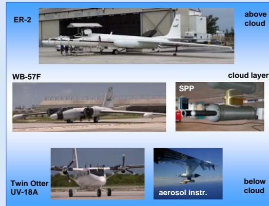
Fig. 2: Research aircrafts participated on CRYSTAL-FACE. ER-2 and Twin Otter measuring solar irradiances above respectively below the cloud and WB-57F measuring cloud microphysics in the cloud layer. Additionally the SPP mounted on WB-57F and the aerosol instrument on board of the Twin-Otter is shown.
