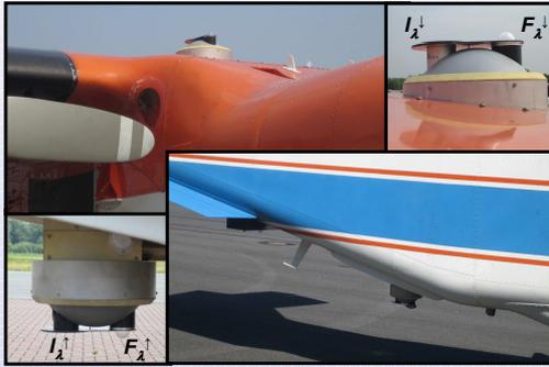
Fig. 1: The SMART-Albedometer mounted on the Polar 2 research aircraft. Close-ups show the optical inlets for irradiance  $F_{\lambda}^{\downarrow}$  (transparent semi-spheres) and radiance  $I_{\lambda}^{\downarrow}$  (flat opening). The grey cupola holding the inlets is automatically tilted for fast and accurate horizontal stabilization during flight.
