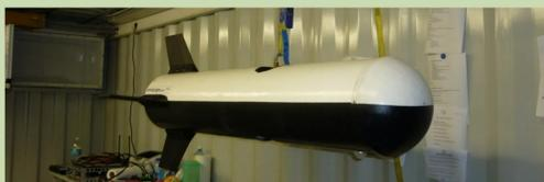
Photo 2: SMART-HELIOS instrument during pitch/roll angle calibration. The platform is attached via a gimbaled mounting.
