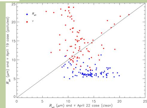
Fig. 8: Retrieved cloud optical thickness  $\tau$  and effective droplet radius  $R_{eff}$  on 19 April 2011 (total aerosol concentration of  $710 \text{ cm}^{-3}$ ) as a function of retrieved results on 22 April 2011 (total aerosol concentration of  $125 \text{ cm}^{-3}$ ). Each data point represents the mean within a 0.01 LWC bin (e.g. within a LWC-range  $LWC = 0.2 - 0.21 \text{ g m}^{-3}$ ). LWC data is from the PVM-100A on ACTOS.
