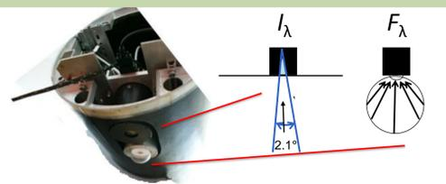
Fig. 3: Radiance and irradiance sensors at the bottom of SMART-HELIOS.
