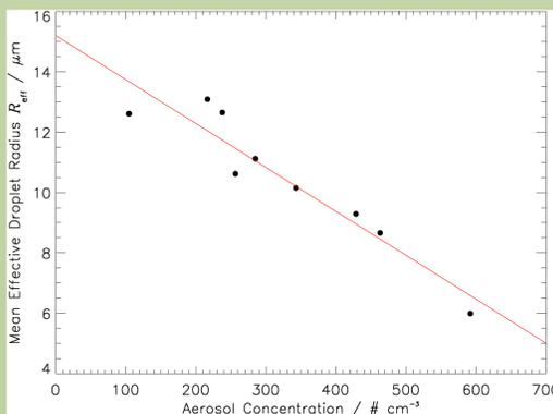
Fig. 7: Retrieved daily mean values of effective droplet radius  $R_{eff}$  as a function of total aerosol concentration data from the CPC on ACTOS. Data is from April 2011. The red line indicates a linear fit through the data.
