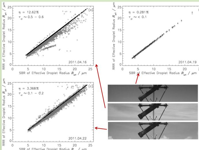
Fig. 6: (a) Radiance-Ratio Retrieval (RRR) as a function of Standard Bi-Spectral Retrieval (SBR) of the effective droplet radius  $R_{eff}$  on 16 April 2011. (b) RRR as a function of SBR of  $R_{eff}$  on 19 April 2011. (c) RRR as a function of SBR of  $R_{eff}$  on 22 April 2011.
