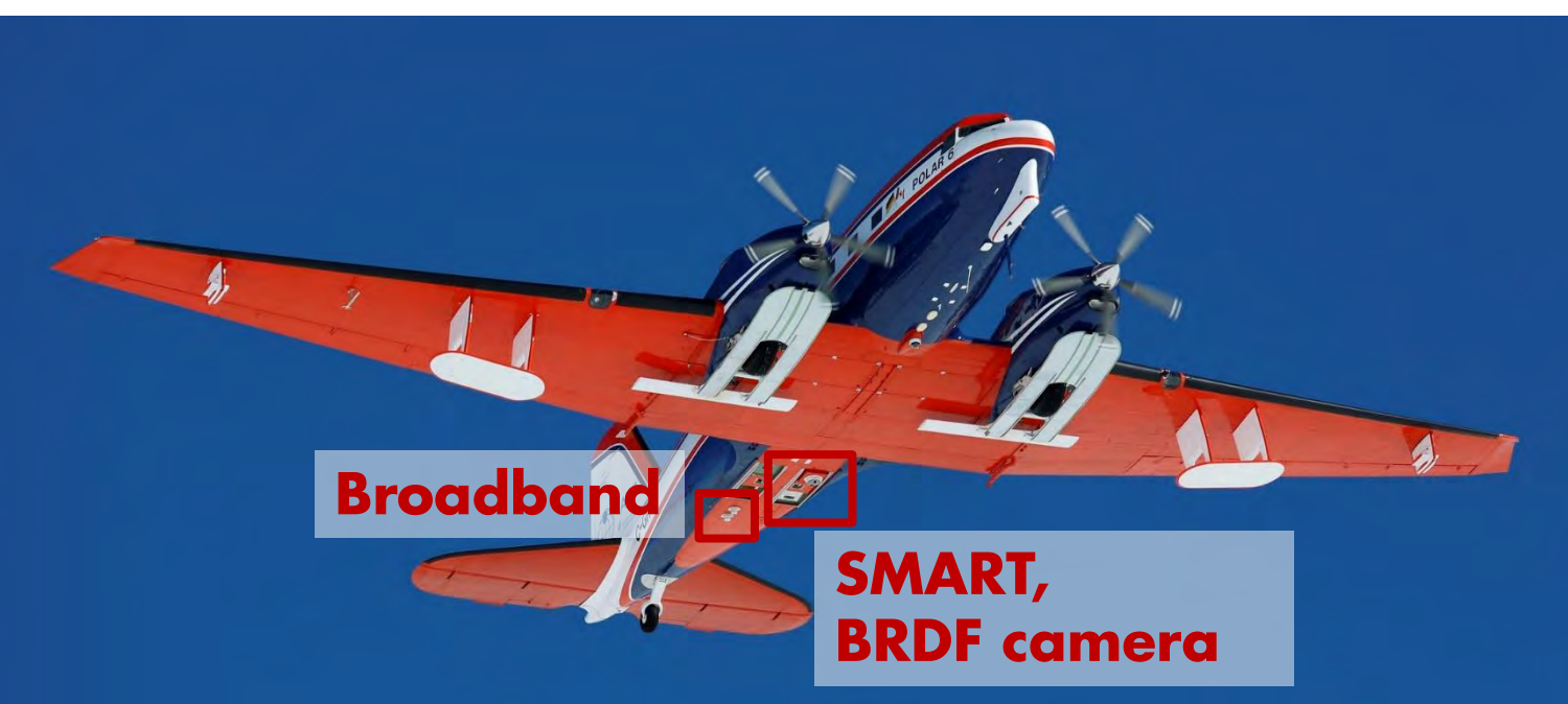
Figure 5: Overview of the instrumentation during ANT-Land 2013/2014 on Polar 6 research aircraft (left) and Kohnen station (right)
