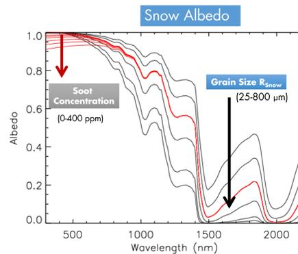
Fig. 2: Simulated spectral snow albedo in dependence of grain size and soot concentration.
