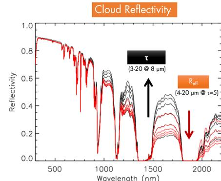
Fig. 3: Simulated spectral reflectivity of a cloud over snow in dependence of cloud optical thickness and cloud particle size.
