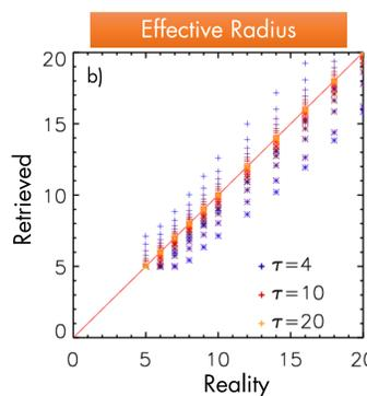
Fig. 5: Comparison of retrieved (synthetic data) and real cloud optical thickness (a) and droplet effective radius (b) when snow grain size is overestimated with 200 μm compared to reality with 50 μm (plus symbols) or underestimated with 50 μm compared to reality with 200 μm (asterisks).
