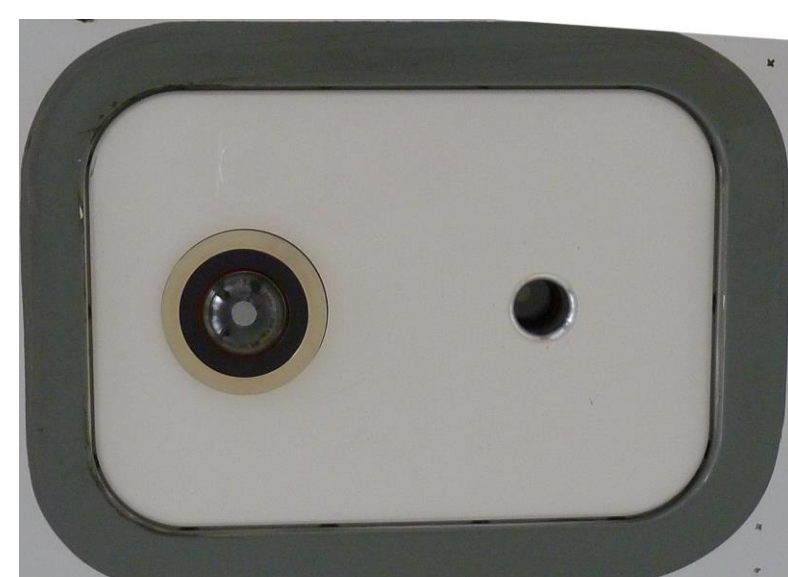
Fig. 2: Location of the HAMP radiometer + radar and SMART optical inlets.
